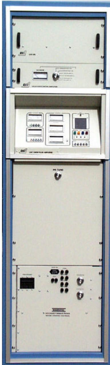
The anode power supply develops 6400 Volts for the PA and 3200 Volts for the IPA. The amplifier is completely protected against IPA and PA anode and grid overloads along with VSWR and over temperature faults. Safety interlocks are located on all compartments where high voltage may be exposed.
