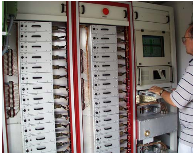
20 KW, 27 mHz, Solid-State Trailer Mounted (Mobile) Generator designed and built for KAI Technologies
